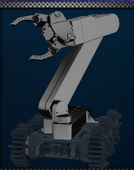
DS4-MS manipulator shown on Macro USA Scorpion SUGV
